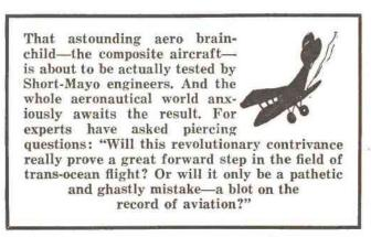
for Atlantic round trips. But once they had figured out the size and details of the craft, they immediately sensed that the weighty ship they had in mind would never be able to get off the water by ordinary means when fully fueled. Thus they hit upon the idea of a special large and powerful ship fitted to carry the real trans-ocean plane in pick-a-back fashion. You might term it a motherand-offspring combination. And "offspring" is decided-
