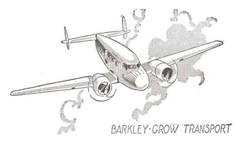
Barkley-Grow wing structure is its multi-spar system and stressed-skin covering. This makes for a particularly rigid airfoil. The center-section portion is part of the fuselage; the outer portions are bolted on, and the wing-tip sections are removable. It is believed that this type of wingdesign is especially staunch against machine-gun fire.
