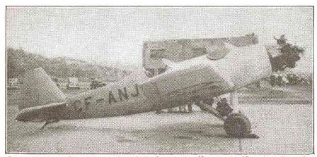
German amateur pilots go strong for this Junkers Junior. Nor can you blame 'em-for such a neat dual-control two-placer would "rate" on any man's light plane tarmae. An all-metal low-wing, it employs the 85-h.p. Siemens-Halske radial. Yes, its striking pursuit-ship lines remind us of our own dushing Ryan S-T.
