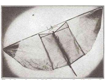
Where's the prop? you ask. Well, there isn't any! For while this peculiar Ledman-Orthof device uses rubber for power, the motor actuates the wings instead of an air-screw. Notice here how simply the framework is built. Ordinary tissue is the covering.
