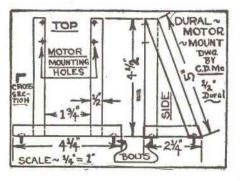
back of the two sides. Solder another piece of the same length to the bottom and back. This piece will have to be bent to a more acute angle to fit the bottom bracers. Make sure that about 1" protrudes on each side of the mount, on both the top and bottom back cross-pieces.
